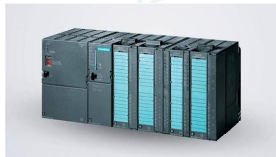
Fig. 1: The Siemens Simatic S7-300 PLC (CPU 315), equipped with a 24 V power supply and four I/O modular units. This is exactly the PLC model hunted by Stuxnet.
