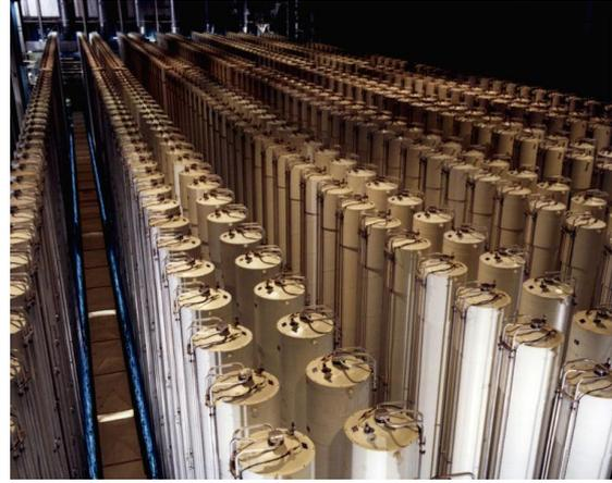
*Fig. 20: Cascades of gas centrifuges in a US fuel enrichment plant in Piketon, Ohio.*
