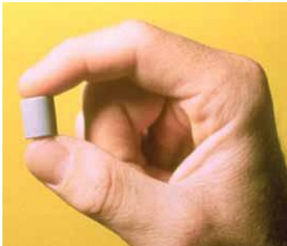
Fig. 19: A uranium dioxide fuel pellet (7 g.). Five fuel pellets meet the electricity needs of a household for one year. A large Westinghouse pressurised water reactor contains 193 fuel assemblies, nearly 51000 fuel rods and approximately 18 million fuel pellets.
