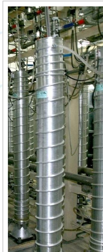
Fig. 6: An IR-1 centrifuge in Natanz. It is essentially a replica of a P-1 Pakistani centrifuge. Consisting of a two metre-long aluminum rotor, it can rotate at peripheral speeds of up to 350 metres per second, equivalent to 1260 km/h (close to the speed of sound).
