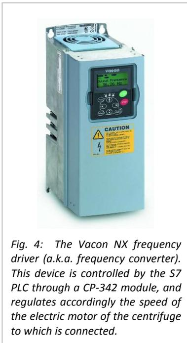
Fig. 4: The Vacon NX frequency driver (a.k.a. frequency converter). This device is controlled by the S7 PLC through a CP-342 module, and regulates accordingly the speed of the electric motor of the centrifuge to which is connected.
