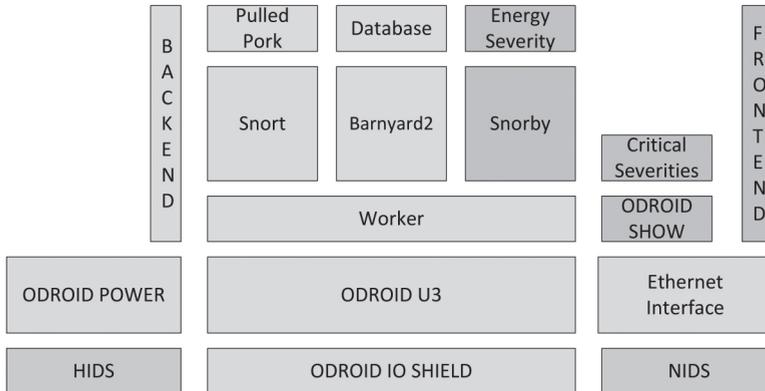
The described architecture can also be operated as HIDS to perform current-based intrusion detection for itself: the main operational mode is the application as NIDS, providing current-based intrusion detection for one or multiple systems by using current-sensing information, but HIDS and NIDS can be operated simultaneously for a current-sensing IDS with permanent self-monitoring.
