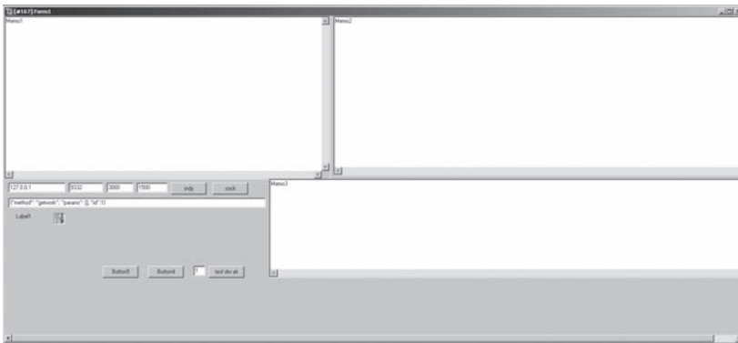
FIGURE 2. A RUNTIME INVISIBLE GUI IS THE BASIS FOR FUNCTIONAL COMPOSITION OF SEVERAL MODULES, HERE FOR A BITCOIN MODULE (CLIENT_8.EXE). EXTRACTED WITH INTERACTIVE DELPHI RECONSTRUCTOR [16].
